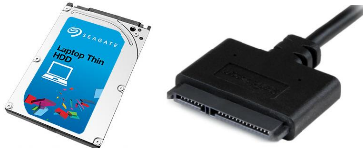
Figure 4: Connecting the SATA connector on the cable to the self-encrypting drive.
